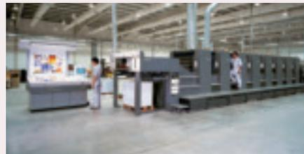
Our presses are connected with TECHKON and XRITE inline print density control systems for closed loop colour control to maintain colour density to FOGRA standards throughout the print run. All our presses are connected with Pre-press to receive CIP4 files for precise colour setting and job details. They are also connected with our Technique MIS system to plan and monitor the production schedule and optimise the whole printing process.
